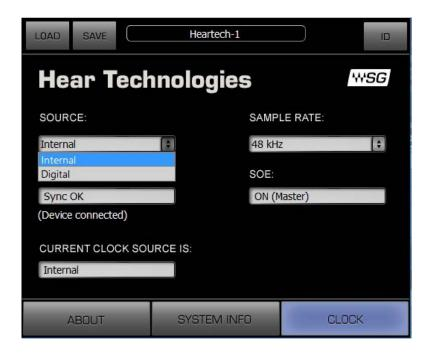
**SAMPLE RATE** sets the sample rate when Clock Source is set to Internal.
