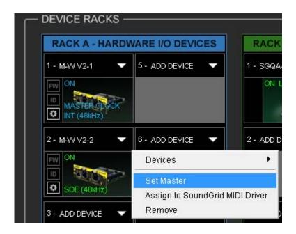
Now you know how to assign I/O devices and designate a device as the clock master. Click on the **Gear** symbol in the device slot to open the Hear Back PRO SoundGrid Card control panel in order to set up clock details and configure preamps.
