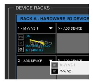
To add another SoundGrid device, click on the arrow in an empty rack slot. From the list of available devices, choose the one that you want to add—in this example, an M-Waves card. In this image, the first I/O device is grayed out (and therefore unavailable), since it is already claimed.
