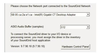
Pressing the "Hardware Control Panel" button on the Driver Control Panel app will open the control panels of all I/O devices assigned to your SoundGrid application. If none are assigned, nothing will happen.
