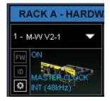
Click on the FW button to launch the Reflasher. This will initiate a scan of the hardware and then offer options. Do not disconnect device or turn off your computer until you see "Done."
