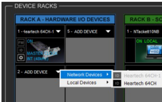
Clock Master Rack Slot 1 and Adding another SoundGrid Device
