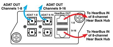
NOTE: The HearBus connections are not Ethernet and are not compatible with the Hear Back PRO HBUS or any Hear Back PRO equipment. HearBus connections are only for connecting to the original Hear Back system. Only the HBUS connections on the Hear Back PRO Hub are used for connecting to other Hear Back PRO Hubs.
